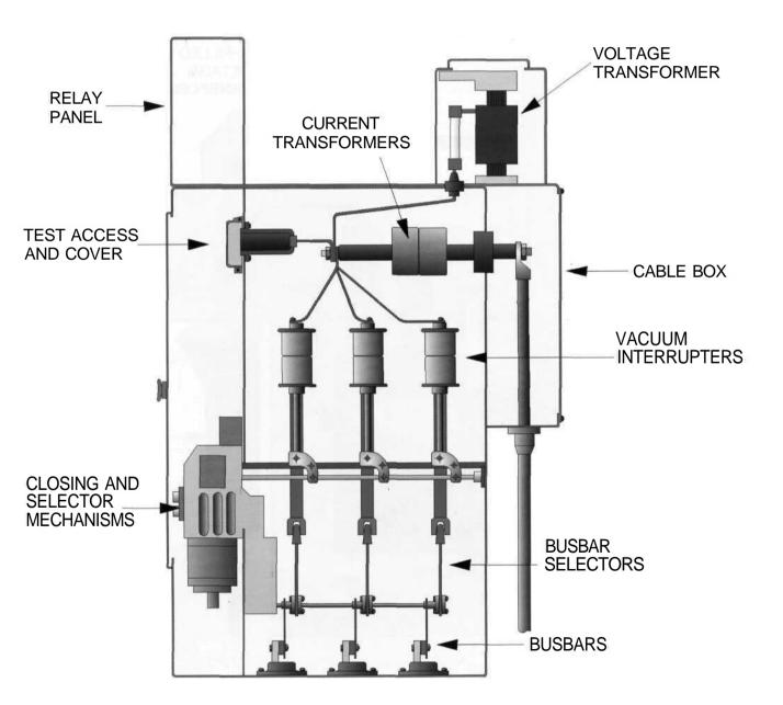
Appendix C4: **Typical arrangement of an 11 kV oil switch**
