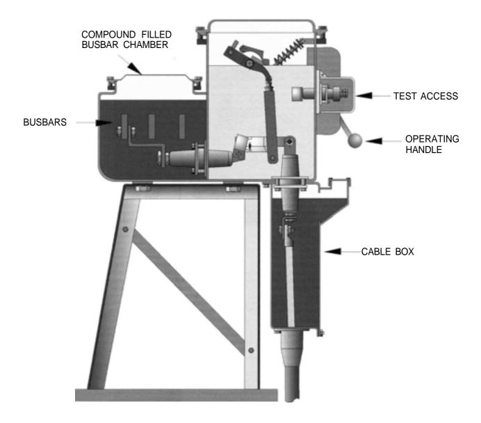
Appendix C5: Typical arrangement of an 11 kV oil fuse switch
